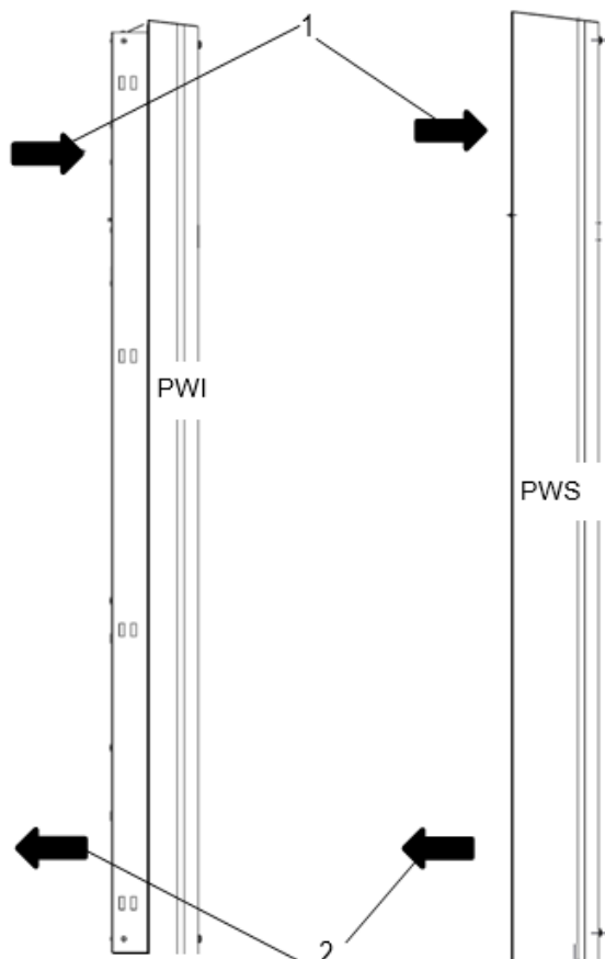
Figure 1 - Side view of air current principle PWI/PWS air/water heat exchangers
